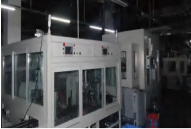
Soundproofing Covers for Equipment
